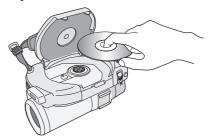
Push the section marked "PUSH CLOSE" on the cover of the disc compartment to close the cover.
